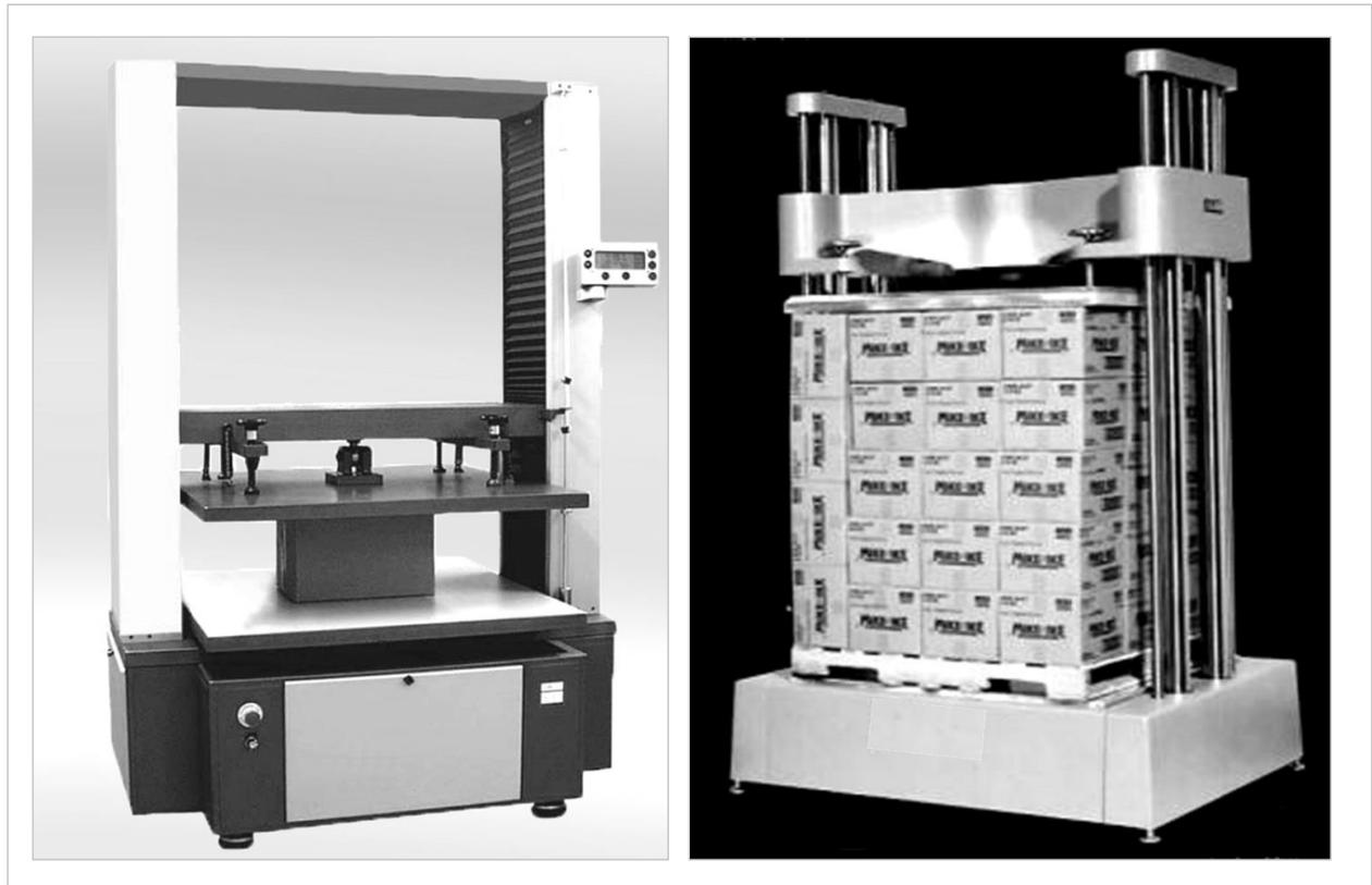
*German Standard DIN 55440-1 Packaging Test; compression test; test with a constant conveyance-speed*
