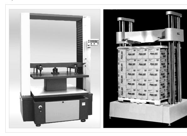
German Standard DIN 55440-1 Packaging Test; compression test; test with a constant conveyance-speed
